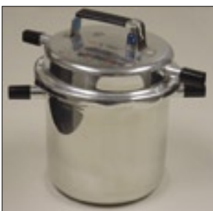
FIGURE 17. Autoclave: high-pressure, saturated steam sterilization
