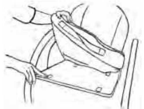
Fig. 2.9. Seat with detachable cushion
