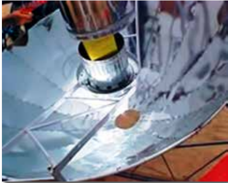
Figure 5.7 Solar melter and safety box of molten syringes
