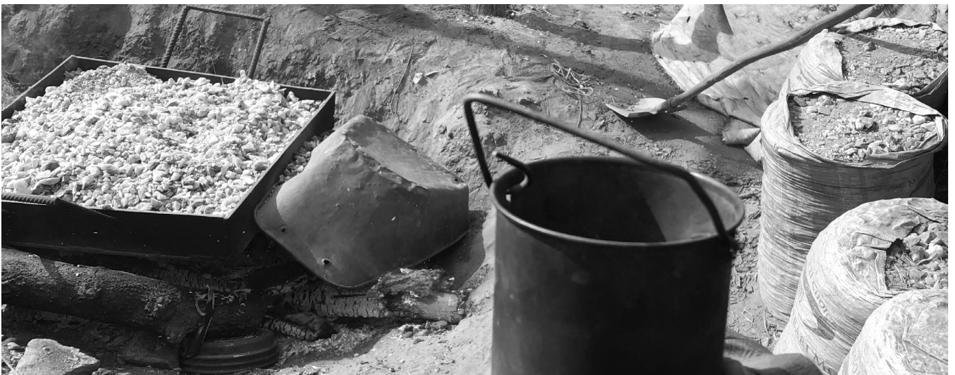
Figure 17: Cup where amalgam is placed and heated to vaporize the mercury (open burning)
