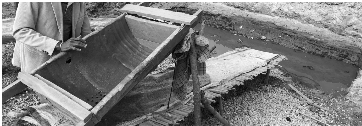
Figure 11: Tools for gold concentration and retention in mesh-net
