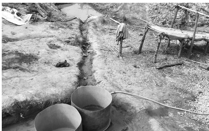
Figure 12: Mercury contaminated tailings in unsafe retention ponds being collected for transportation to cyanide leaching site
