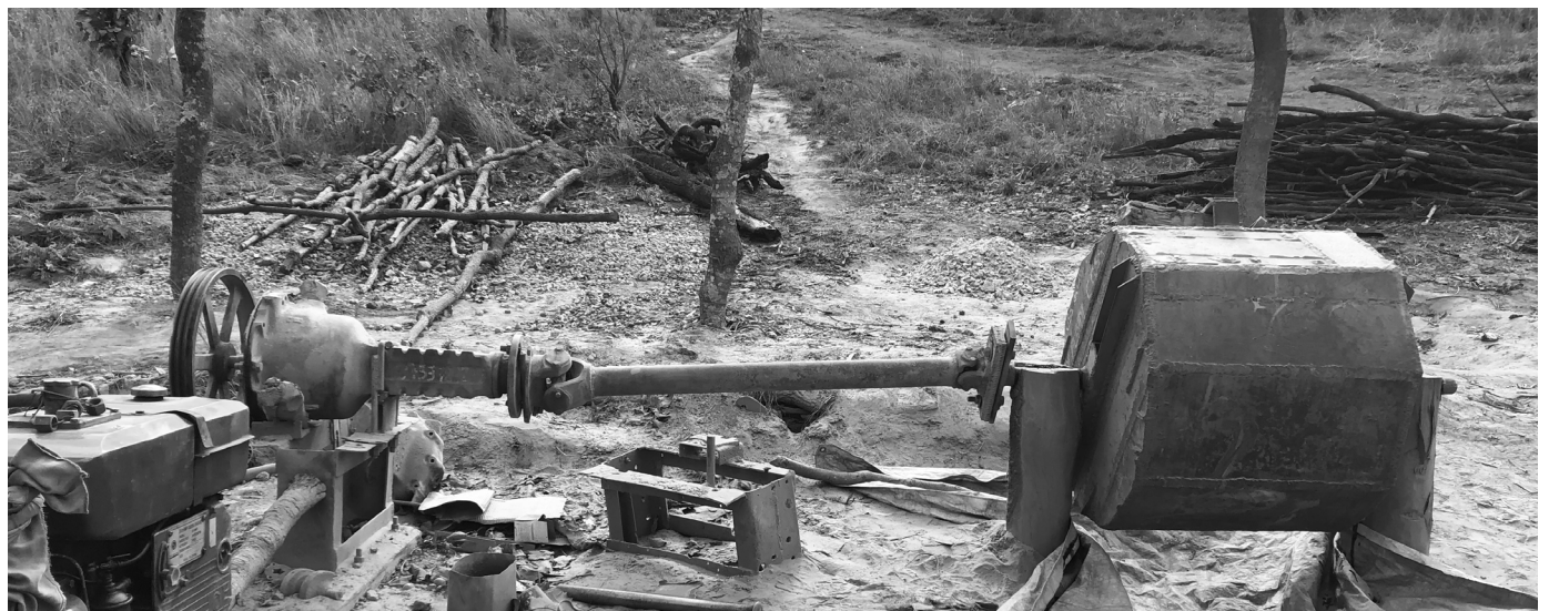
Figure 10: Mill for crushing ore into fine powder
