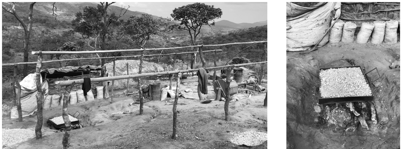
Figure 9: ASGM site where processing, concentration, amalgamation and burning take place (left) and heating crushed ore before milling (right)
